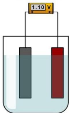
An electrochemical cell consists of two metals of **different reactivity** dipped into an **electrolyte**.
