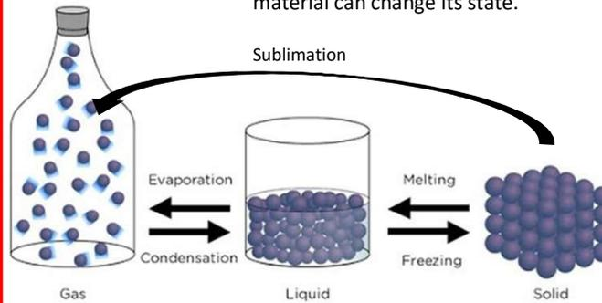
**Specific latent heat** → The amount of energy required to **change the state** of **1kg** of substance **without changing the temperature**.
