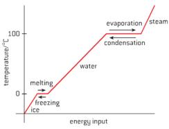
The horizontal parts are caused by energy being needed to break bonds and change state .i.e. move from solid to liquid to gas.
