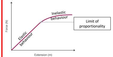
Work is done when a spring is extended or compressed. Elastic potential energy is stored in the spring:
