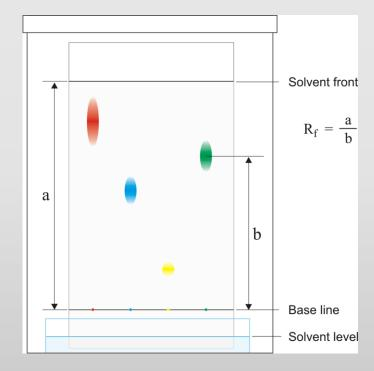
$$R_f = \frac{distance \ moved \ by \ substance}{distance \ moved \ by \ solvent}$$
